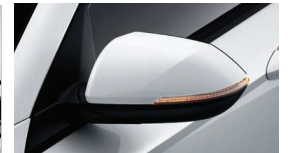
Outside mirror (Heated / Folding / Turn signal indicator LED)
